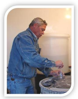
Water Production Operator Bill Kline tests the strength of chlorine which is used in one of our many district well sites.
